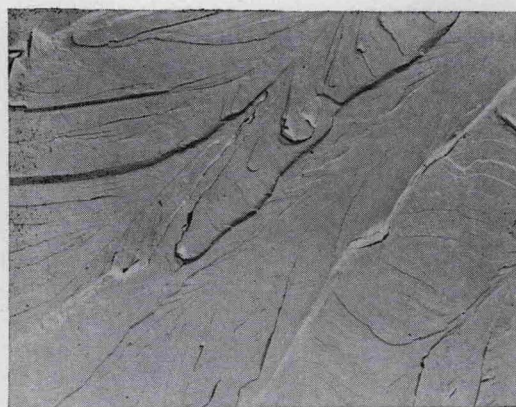
FIG. 3. The appearance of the fracture surface of a pure bismuth specimen which fractured at 5.0 \times 10^8 \text{ N/m}^2 . 3250 \times
